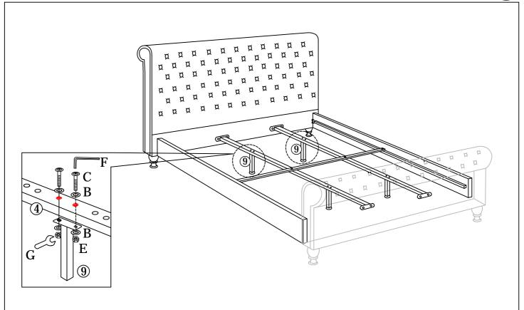
Align the pins on the Holders to the holes along the Centre Rail and the Siderails. Gently tap them into the holes using hand palm.
