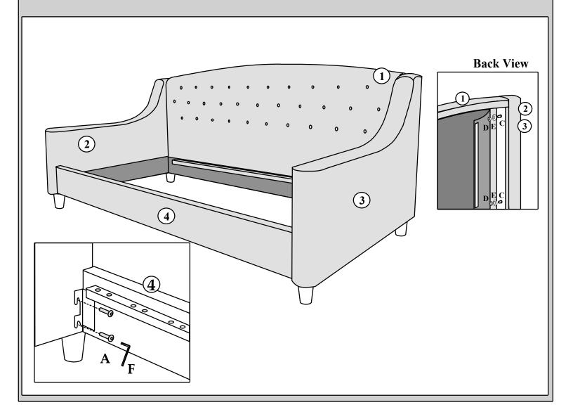
3 Secure the back panel as shown in diagram. Attach across rail to the base.
