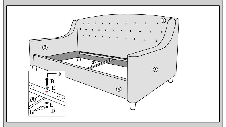
Align the pins on the Holders to the holes along the siderail and back panel. Gently tap them into the holes using hand palm.
